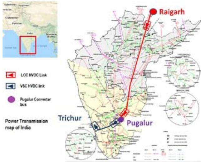
**Fig. 1 :** Raigarh-Pugalur-Trichur HVDC Transmission Scheme in Southern Region of India<sup>[2]</sup>
