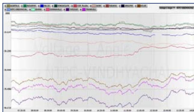
Fig. 1 : Angular separation monitoring of various nodes in the Indian grid with respect to one node from the WAMS system
