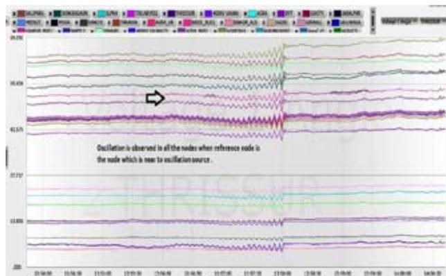
Fig. 11 : Wide area angular separation when the reference node is selected near to the source of LFO
