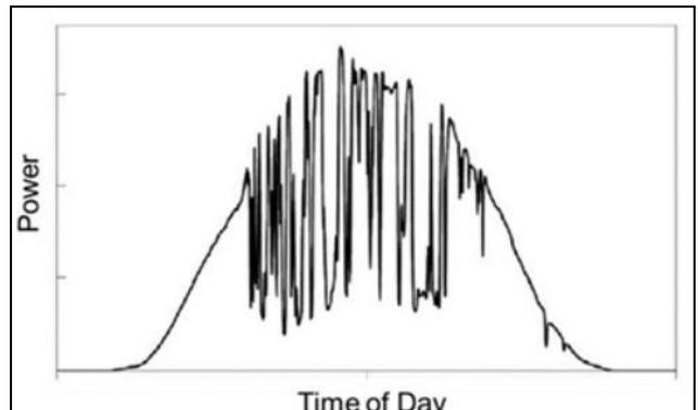
Fig. 4 : Power output from solar during a typical summer day having random cloud cover
