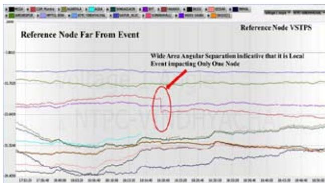
Fig. 8 : Wide area angular separation when the reference node selected far from the event/disturbance location
