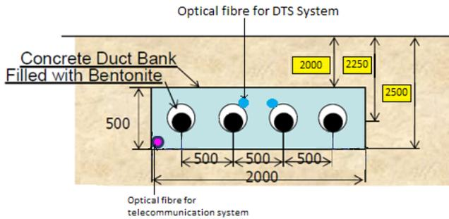
Typical HVDC cable & Fiber Optic in Duct bank
