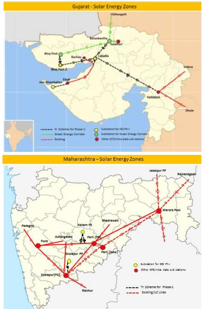
**Fig. 7 :** Transmission scheme for renewable energy zones in Gujarat (Ph-I: 6 GW) & Maharashtra (Ph-I : 3 GW)
