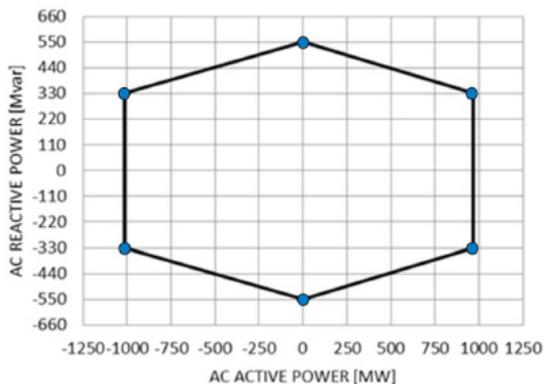
The above capability requirements are valid for AC system voltage between 380-420 kV. If AC voltage is outside this range then restrictions at some point may appear. The capability of converter varies based on following factors- AC system voltage, frequency and DC voltage.
