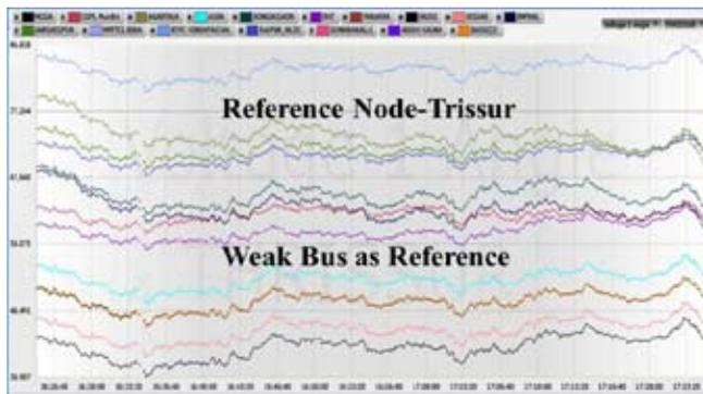
**Fig. 3 :** Weak Bus/Node in SR grid used as a reference for Wide Area Angular Separation Monitoring
