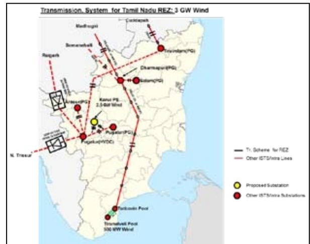
**Fig. 9 :** Transmission scheme for renewable energy zones in Tamil Nadu (Ph-I : 3 GW)
