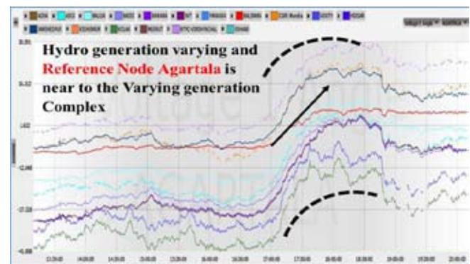
Fig. 10 : Wide area angular separation when the reference node is selected Near to the varying generation complex
