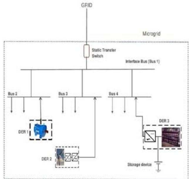
Fig. 1 : Single Line Diagram for Typical Microgrid
