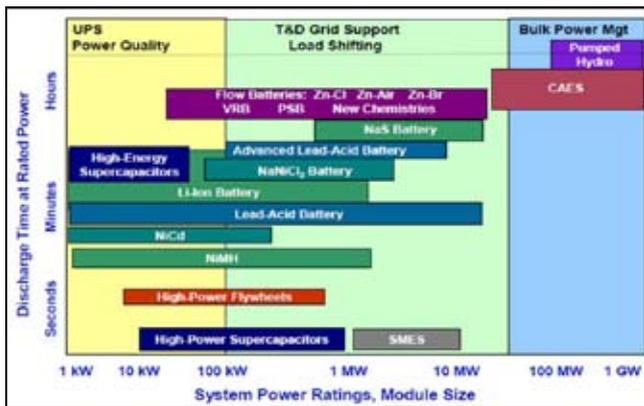
Fig. 2 : Power rating and rated Energy capacity<sup>[05]</sup>
