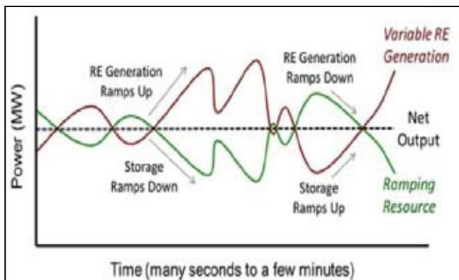
Fig. 5 : Variable RE and Storage Ramping
