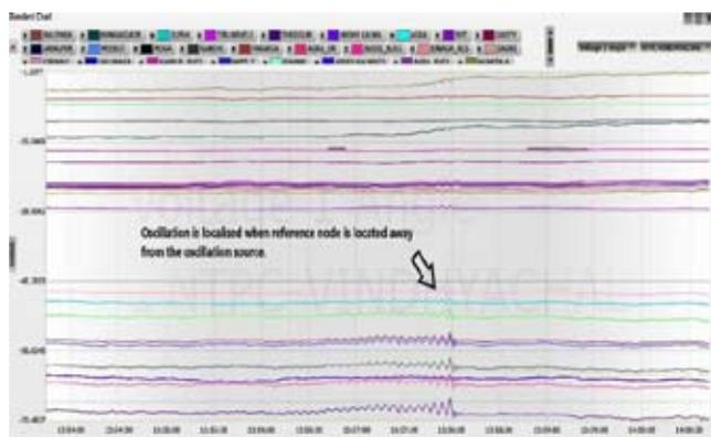
Fig. 12 : Wide area angular separation when the reference node is selected away from the source of LFO
