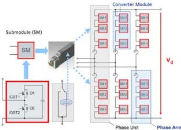
**Fig. 4 :** Typical VSC-HVDC multi-level topology<sup>[4]</sup>
