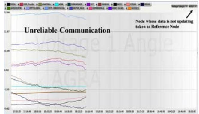
**Fig. 5 :** Reference node selected having unreliable communication causing non-availability of wide area angular separation from all nodes
