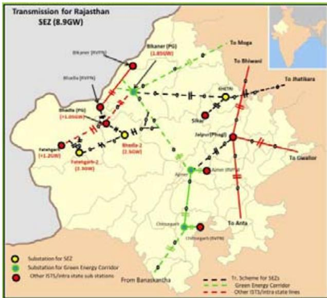
**Fig. 6 :** Transmission scheme for solar energy zones in Rajasthan (Ph-I :8.9GW)
