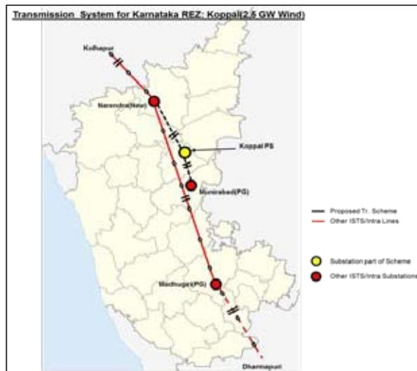
**Fig. 8 :** Transmission scheme for renewable energy zones in AP (Ph-I: 4.5 GW) & Karnataka (Ph-I: 2.5 GW)
