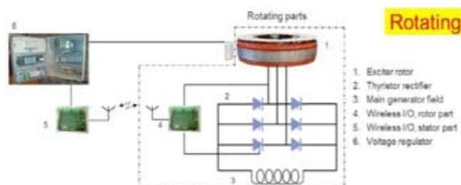
Fig. 1 : Typical arrangement to Use Bluetooth Technology to fire thyristors
