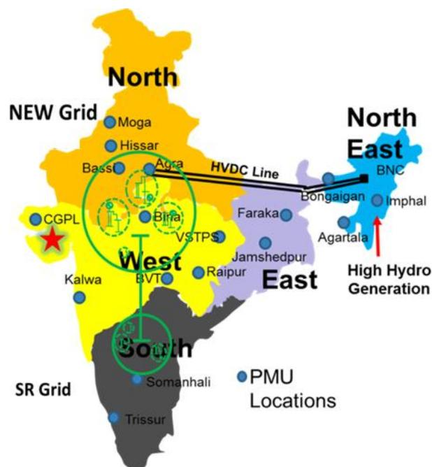
**Fig. 2** : Indian Grid shown as the synchronous interconnection of five regional grids. Nodes with PMU are shown in blue. Node with Event, HVDC Line, Varying High Hydro Generation Complex is highlighted for case studies reference.
