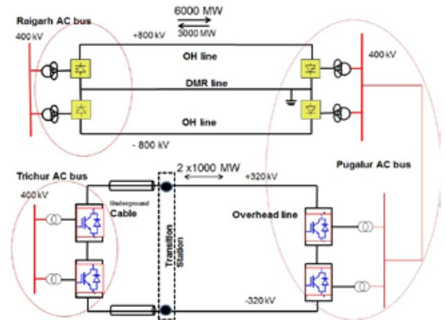
**Fig. 2 :** Common Pugalur Converter bus for Raigarh-Pugalur LCC and Pugalur-Trichur VSC HVDC Links
