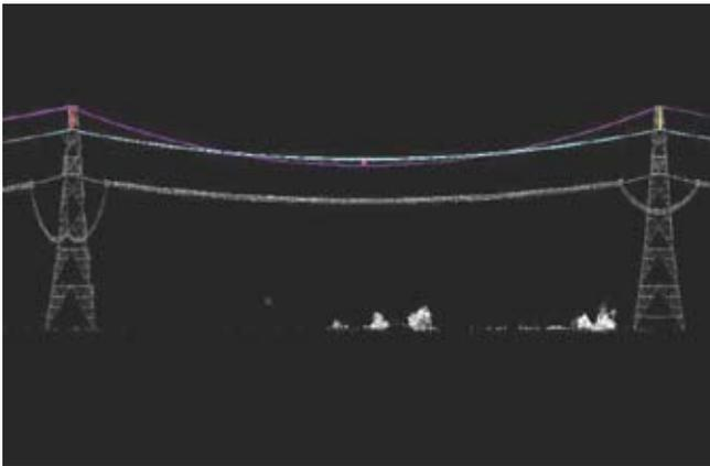
LIDAR image of line indicating high sag in Earthwire
