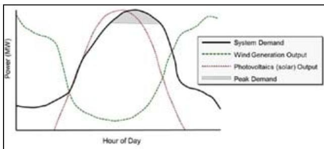
Fig. 6 : Wind and Solar Generation Output and System demand profiles, not including ramping.
